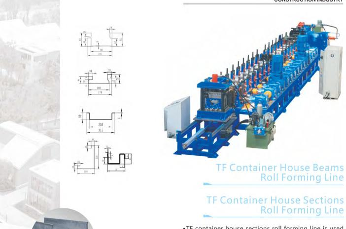
•TF container house sections roll forming line is used to produce sections such as top beam, ground beam, column and flashing gutter for container house production. The production line is equipped with uncoiler, puncher, forming machine, cutting machine, electrical control system and hydraulic system to finish one-time processing.
